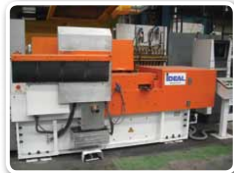
⑤ Flash-Butt Welding VJ is one of the few manufacturers that uses flash-butt welding for joining sleeves and rings together. It involves pressing 2 ends together and running a current between them, forming a seamless joint that is free of oxides. Benefits to customers is a first class coupling with a 'solid-state weld' which will meet the required design life.
