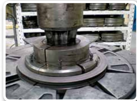
③ The Post Welding Cold Expansion Process Creates dimensionally stable rings of repeatable quality essential for the consistent compression of the annular gasket.
