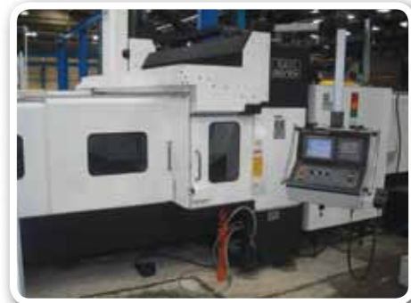
⑥ Vertical Machine Centre This vertical machine centre gives VJ the in-house milling and drilling capability of items up to 2.8m wide. Previously, this process was subcontracted out and took 14 days.
