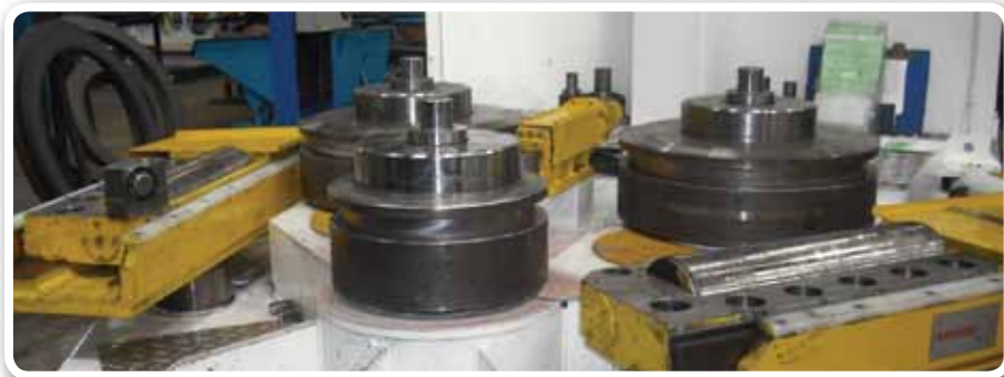
① The Large Ring Bar Bending Machine Can roll bars up to 75mm thick. This has eliminated 90% of segment welding, thereby reducing process time from 1 day to 100 minutes.
